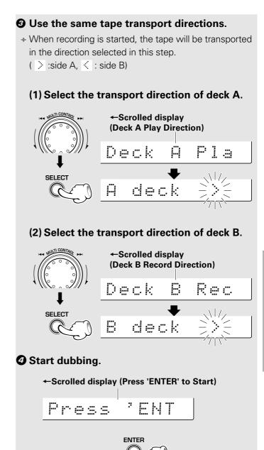
÷ Dubbing ends automatically when the side(s) to be dubbed has been fully recorded on.
